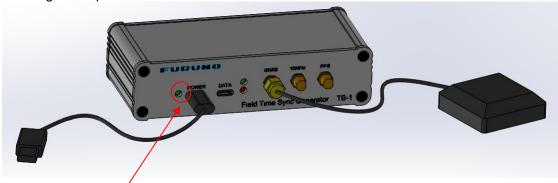
Connect the included USB cable (TypeC connector) to the Power USB jack of TB-1, and TypeA connector to a USB power adapter.
